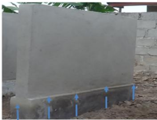
Fig 14. Water observed at height over 320 mm for the CBs
